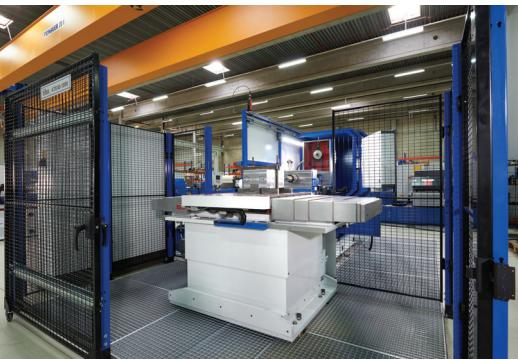
machines will allow high-precision drilling operations with minimal runout in alloys typical for the applications such as nickel steels. The machines come with additional features specially developed for the task, for example chip breakage monitoring for reliable cutting which is integrated as standard.
