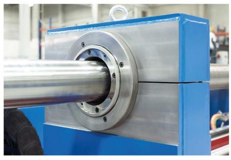
elasticity of the tube, the greater the potential torsional and flexural vibrations. These vibrations need to be minimised as far as possible, as they have a direct effect on the drilling quality and on the operational life of the tool.
